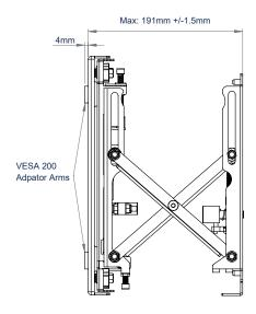
Min: 64mm +/- 1.5mm 4mm **VESA 200** Adpator Arms Interface arms are set at the lowest point. Height adjustment range: 12mm
