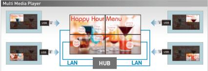
Connecting more than one unit with LAN cable reproduces files in USB memory simultaneously. One of the units becomes Master, and the others Slaves
